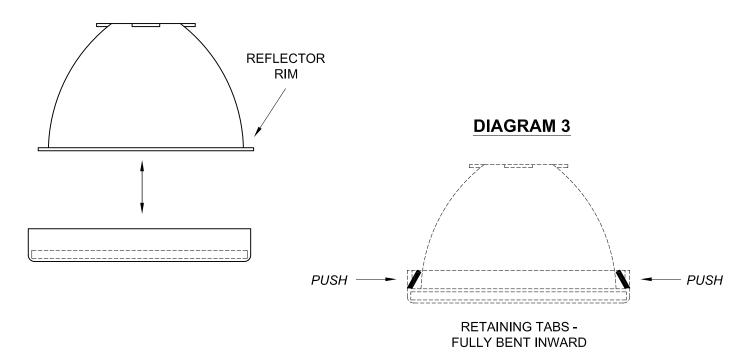
3. Squeeze the two Retaining Tabs inward such that they firmly press up against the side of the reflector and overlap the Reflector Rim. (See DIAGRAM 3)
