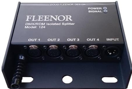
The 124 is an economical bi-directional DMX512/RDM splitter. It is available with 3 pin (model 124-3) or 5 pin (model 124-5) XLR connectors for all DMX512/RDM connections, as well as RJ45 connectors (model 124-RJ) and terminal block connectors (model 124-TB). These splitters have fully isolated inputs. The four outputs are separately driven, but are not isolated from one another.
