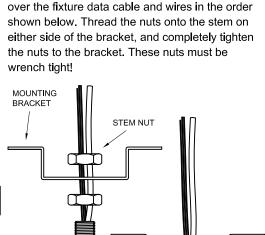
3) Slip two stem nuts and the mounting bracket
