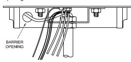
7) Using the terminal block provided, make up the data connections according to list below. CAUTION: If shielded control cable is used, make certain that NO portion of the shield or shield wire (aka drain wire) is bonded to or incidentally in contact with GROUND, or anything electrically connected to GROUND!
