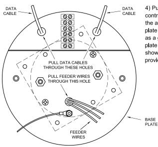
4) Pull the feeder wires and contractor's data cable(s) through the appropriate holes in the base plate using the diagram to the left as a guide, then attach the base plate to the electrical box as shown, right, using the screws provided with the box.
