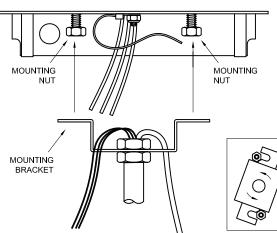
5) Attach the mounting bracket to the base plate by keying the bracket slots between the plate and the two mounting nuts, then tighten the nuts wrench-tight. Use the diagrams, below, and to the left and right as a guide.
