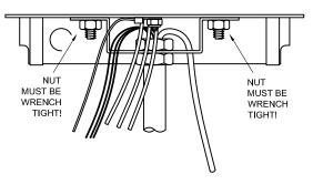
6) Slip the fixture data cable through the barrier opening as shown.
