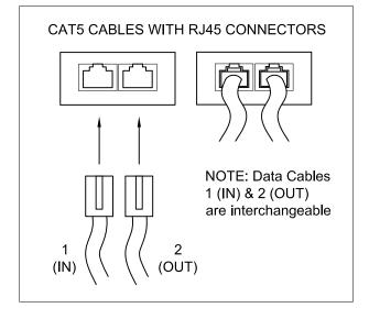
NOTE: The data connector and its connections can be accessed from inside the fixture after the fixture has been installed. Refer to the section titled "SERVICING" in the LINEAR DOWNLIGHT INSTALLATION INSTRUCTIONS that came with the fixture.
